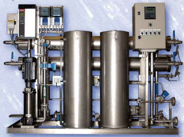
Björk Rostfria ABs AR 3,5/2 is very neat and compact. Measurement 780 mm wide, 2320 mm long and 1820 mm tall. Mounted in our factory and delivered ready to operate.
